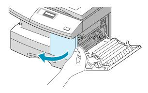
**3** If the cartridge locking lever is on the lower position, turn the lever upward until it locks into place.
